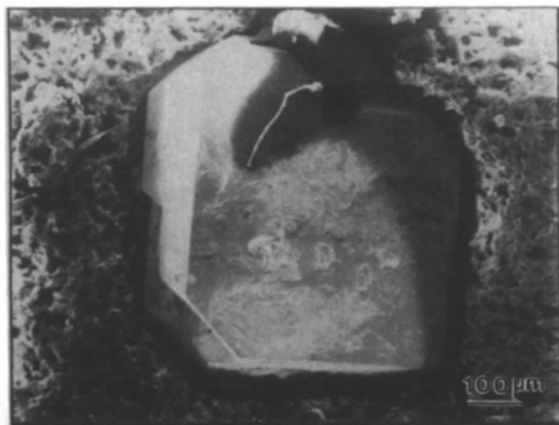
Fig. 2. SEM image of one \text{Al}_3\text{Zr} particle after about 100 h of crystal growth. The magnification is \times 100 .
